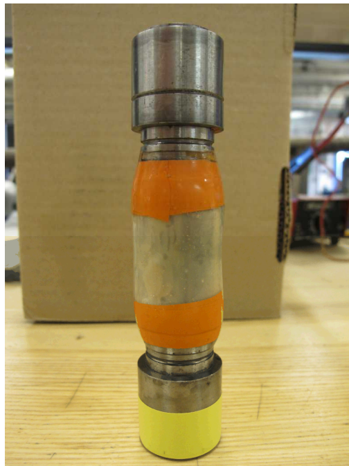
Fig. 3. Image of the jacketed specimen with endcaps.
