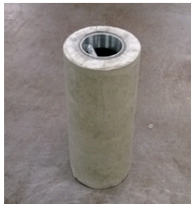
Figure 2 – Specimen with cement sheath cast around a steel casing.
