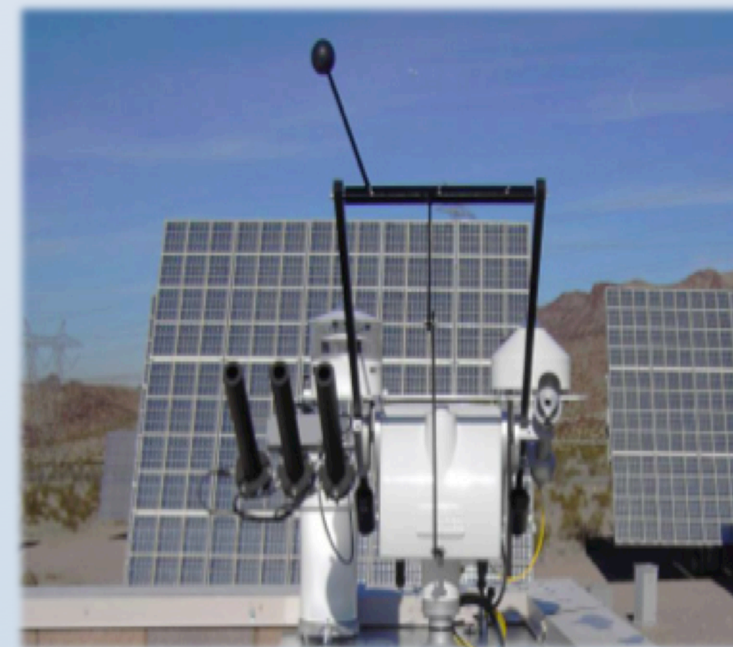
Figure 6. Solar tracker measures direct normal irradiance at the Nevada RTC, with 84kW CPV system in the background.
