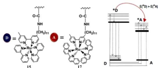
Figure 8. Donor and acceptor monomers used in both ATRP and RAFT polymerization reactions.
