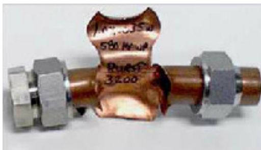
Failure of tubing at 3300 psig water ( above ) and 3200 psig gas ( below )
