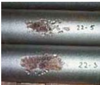
Effects on piping from external corrosion ( above left ) and internal corrosion ( above right ).
