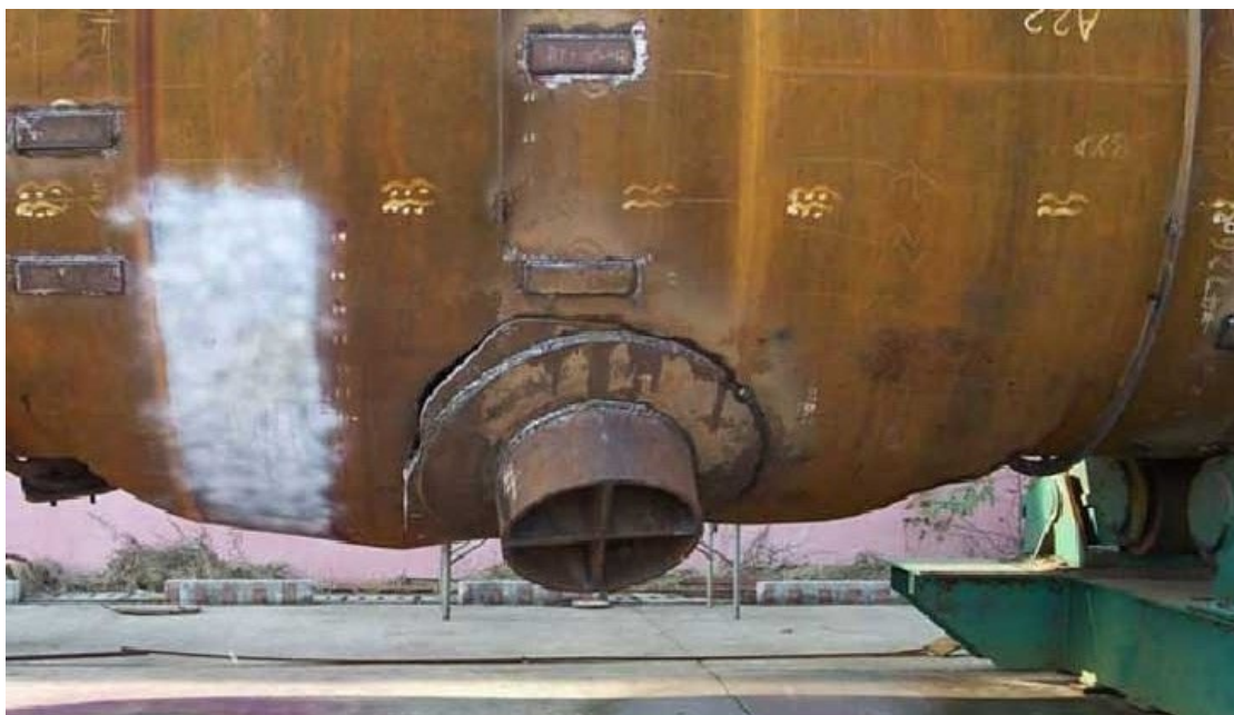
Cracked vessel from a failed hydrostatic test - from www.wermac.org
