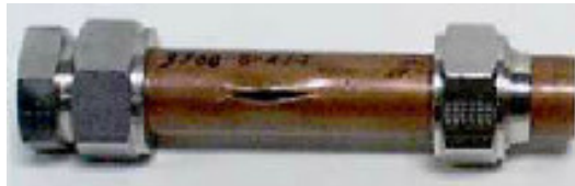
Failure of tubing at 3300 psig water ( above ) and 3200 psig gas ( below )
