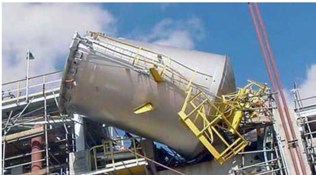
Unexpected result of a pneumatic pressure test on a newly manufactured tank - from www.wermac.org
