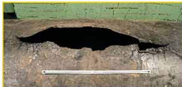
Effects on piping from external corrosion ( above left ) and internal corrosion ( above right ).
