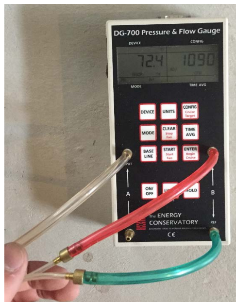
Figure 24. DG-700 used to measure total system airflow
