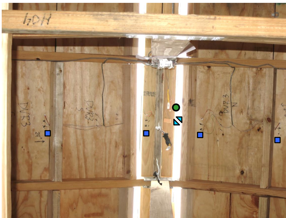
Figure 29. Typical ridge monitoring package with sensors highlighted
