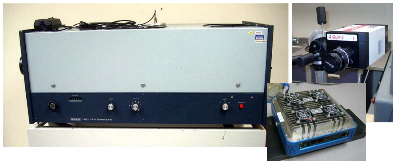
Fig. 4. High resolution spectrometer equipment. Left: 1 m SPEX spectograph, right: detectors – 4QuikE fast camera (upper) and 1024 x 1024 CCD detector (lower).
