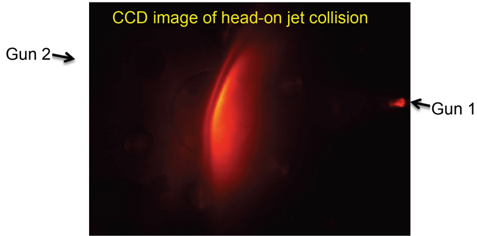
Figure 6.2: Image of head-on collision experiments with argon plasma jets from [28].
