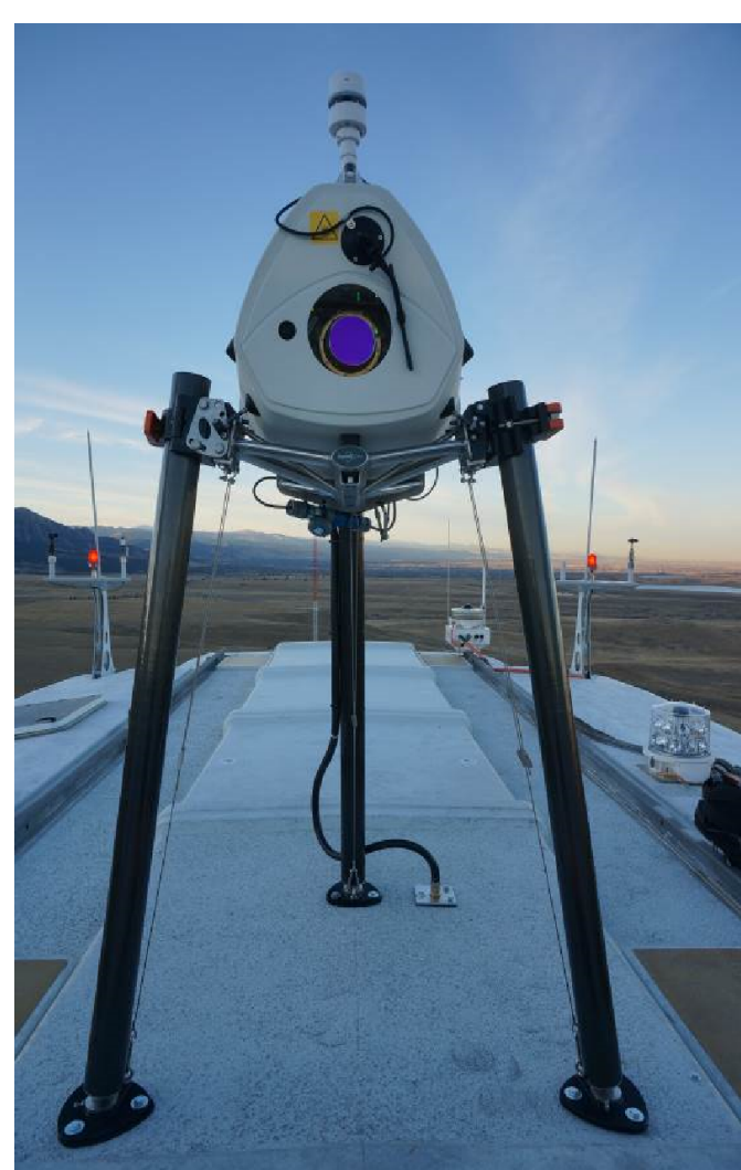
LIDAR installed on ECO110
