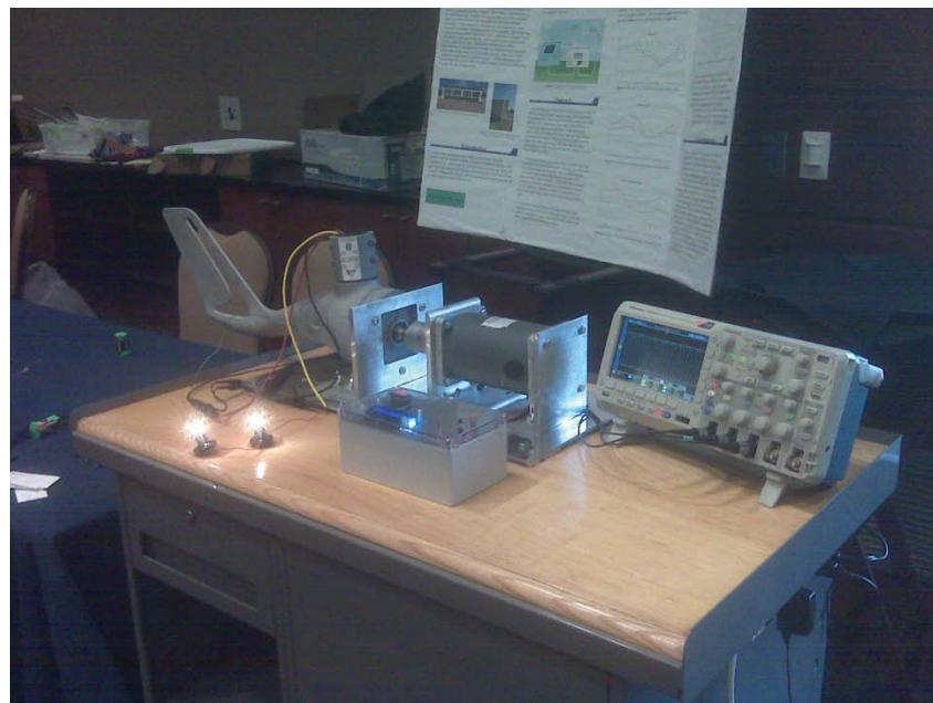
**Figure 3 – Portable Air-X testbench.**
