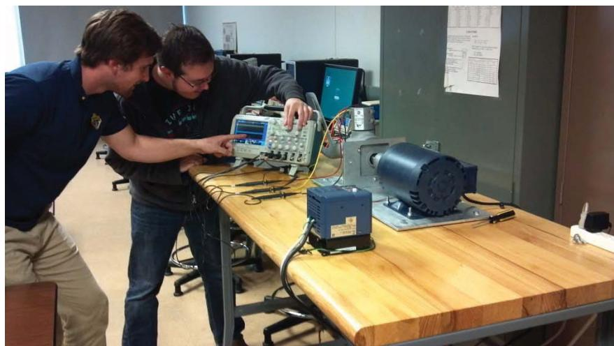
**Figure 1 – Experimental test bench for Air-X wind generator.**
