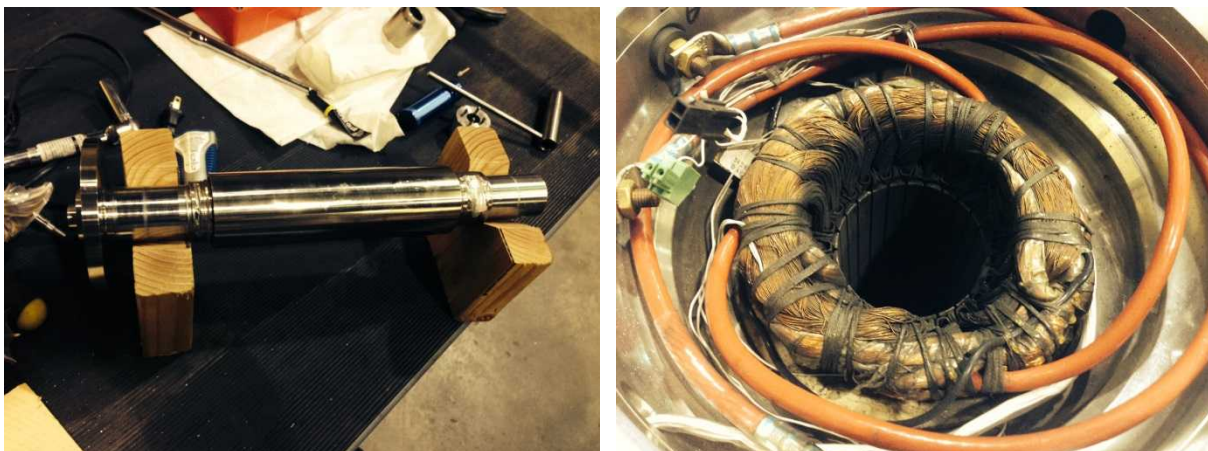
Figure 1. Photos of (left) rotor and (right) stator
