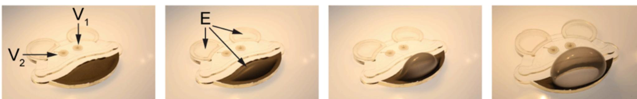
Check valves enable finger-actuated pumping of air and fluid into a "microfluidic frog's" throat. Air moves through the right nostril into the eyes, which are depressed to fill the throat with air. Abbreviations: V<sub>1</sub> = valve 1, V<sub>2</sub> = valve 2, E = elastomeric membrane.
