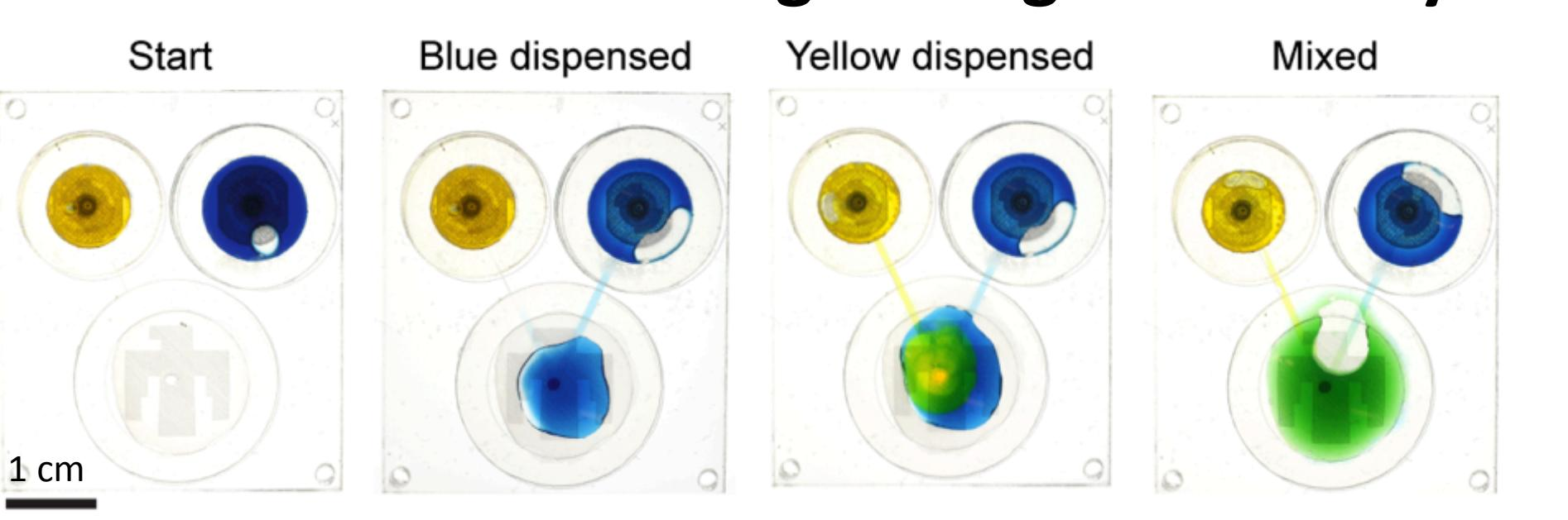
Laser engraved PMMA device with check valves demonstrating finger-actuated, sequential delivery of different fluid volumes to a common mixing chamber.
