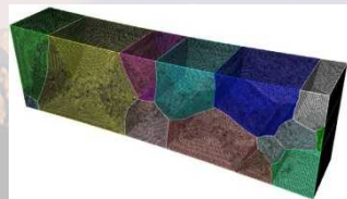
Gauge Section of Oligocrystal Tensile Specimen (1x3x5 mm)
