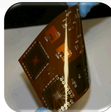
“Flexible Chips” with Printed Wirebonds
