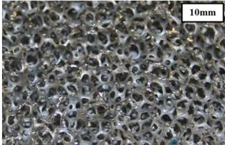
Figure 6–5: Digital image of open-cell Al foam supplied by ERG Aerospace Corporation with 5PPI
