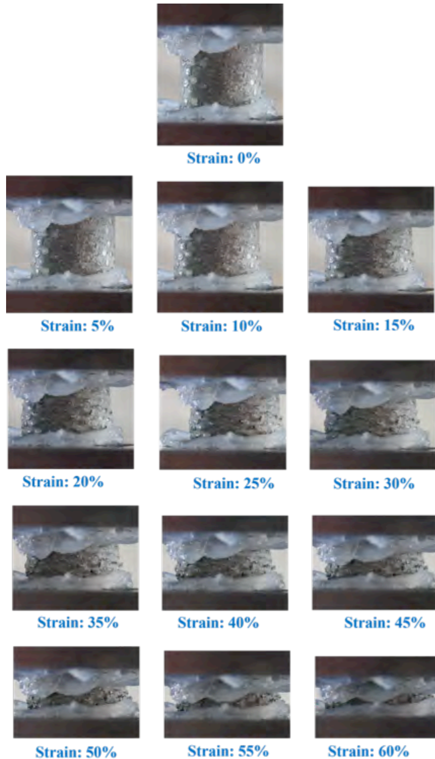
Figure 5–13: Sequential images showing the deformation of (4mm sphere) HZ S-S CMF under quasi-static loading. The white area on the top and bottom are vacuum grease used for lubrication.
