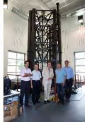
Test section on earthquake shake table
