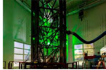
Test section illuminated by 6 PIV laser planes
