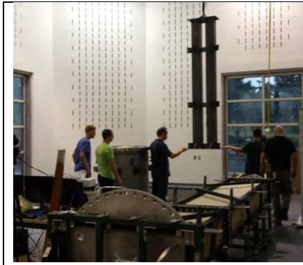
Installation of first columns. Inlet plenum is already in place
