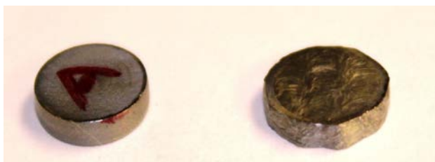
Figure 9. Wrought (Left) and AM (Right) 304L SS Specimens After Testing
