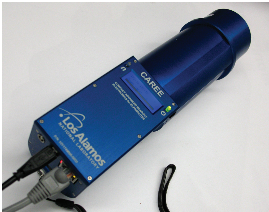
Figure 5: A photograph of CAREE in use. (A USB and Ethernet cable are both attached, although only the Ethernet is required.)
