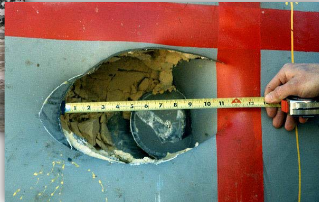
CTU-1 Puncture Drop No. 7; Post-Drop Damage
