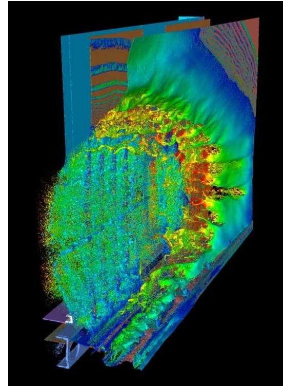
32,000 processor calculation showing nearby blast on aluminum and steel structure
