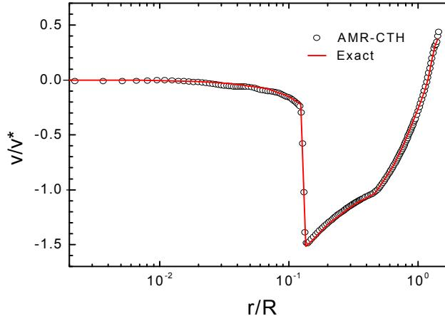
Verification: adiabatic collapse of an initially isothermal spherical gas cloud.
