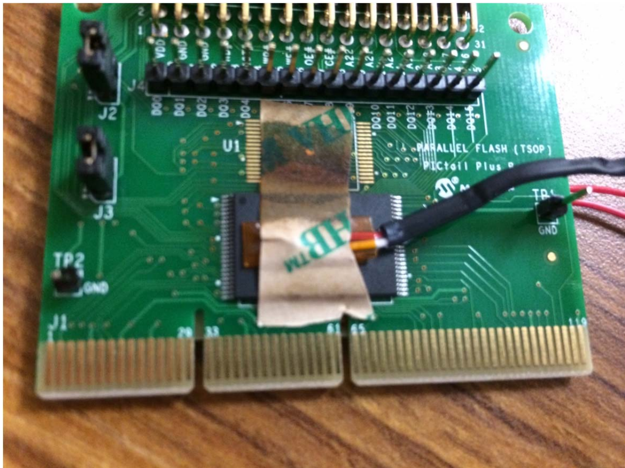
Figure 5. The temperature sensor (an RTD) is directly in contact with the flash memory module on the front side of the board. The two red wires to the resistive heater on the backside of the board can be seen to the right.
