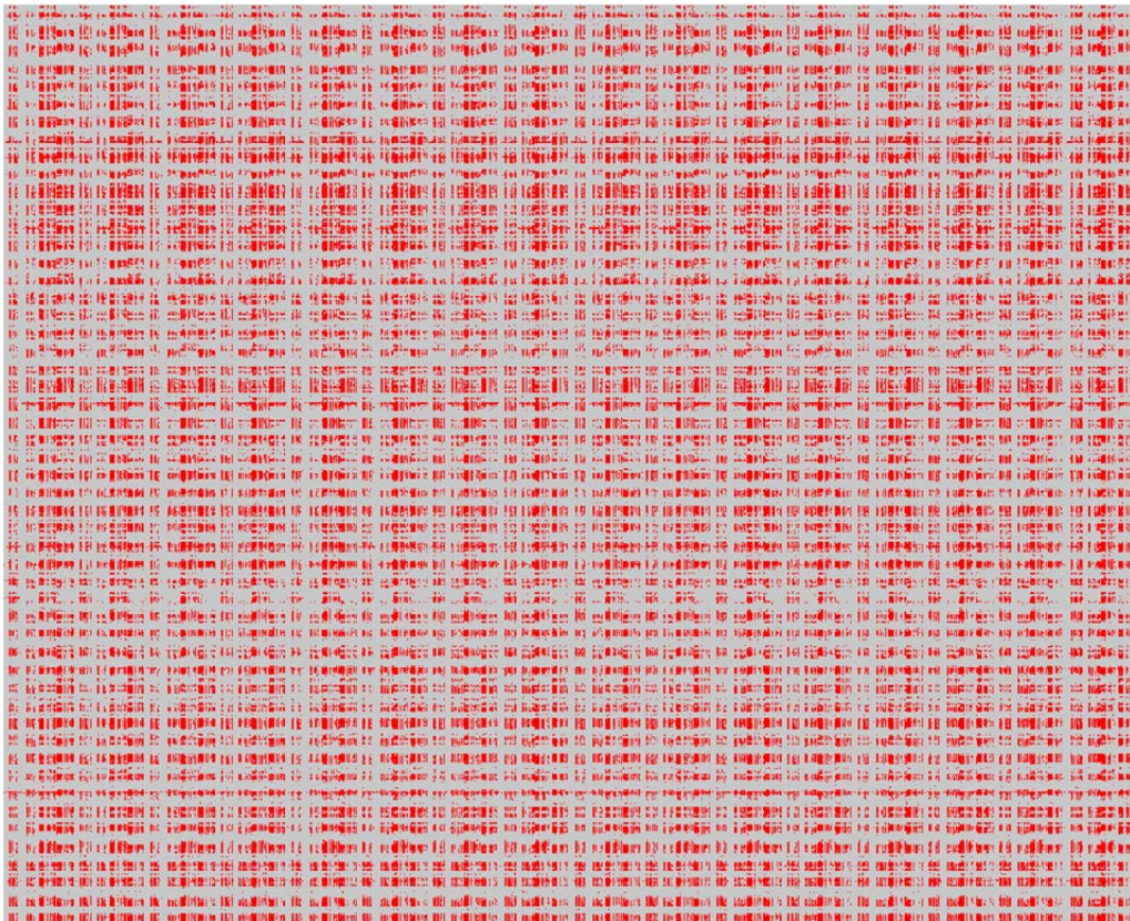
Figure 53. Erase failures (red dots) in second radiation test of ASIC eFlash at dose of 63.7 krad(Si).
