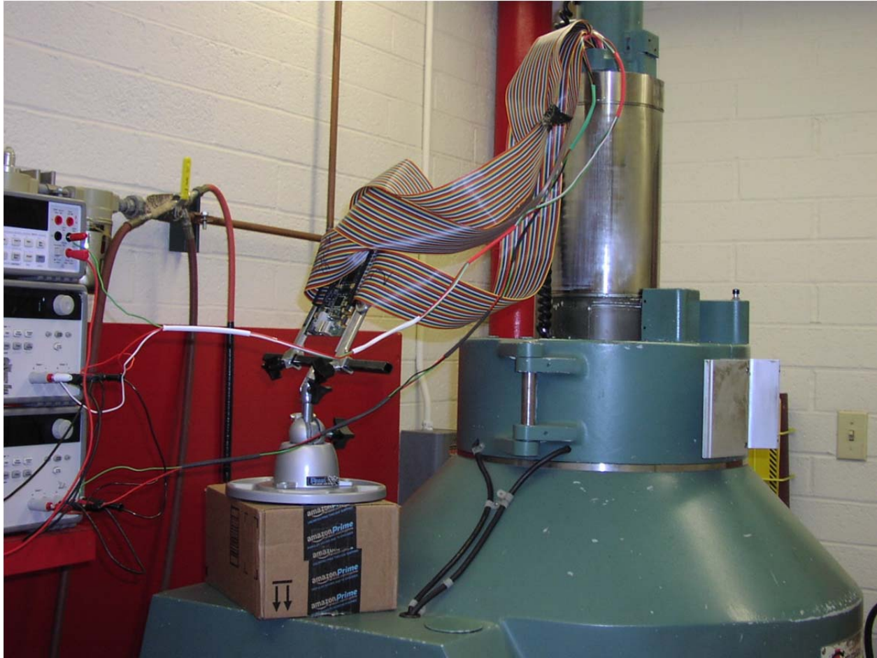
Figure 49. Using four ribbon cables, the FPGA is connected to the ASIC, which has been positioned within the irradiation chamber. Power supplies are located to the left on the red bench.
