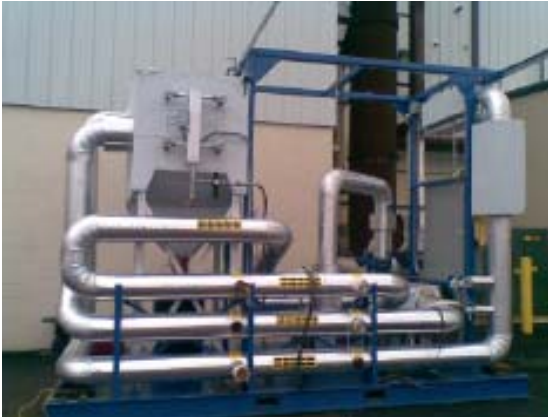
Figure 3-11 Air Liquide's High Performance Dust Filtration Test Skid
