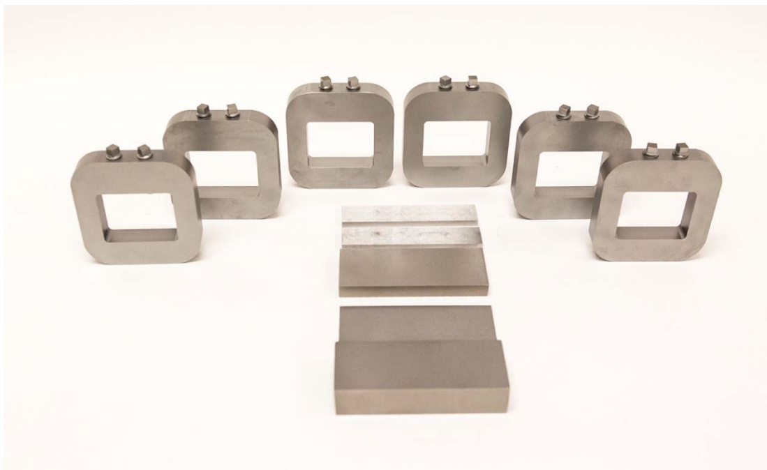
Figure 8. The clamping jig and parts to be bonded.
