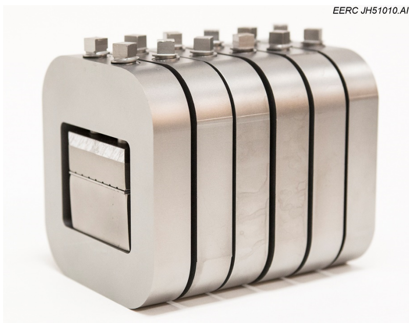
Figure 9. The assembled jig in preparation for heating to bond the APMT plate to the superalloy block.
