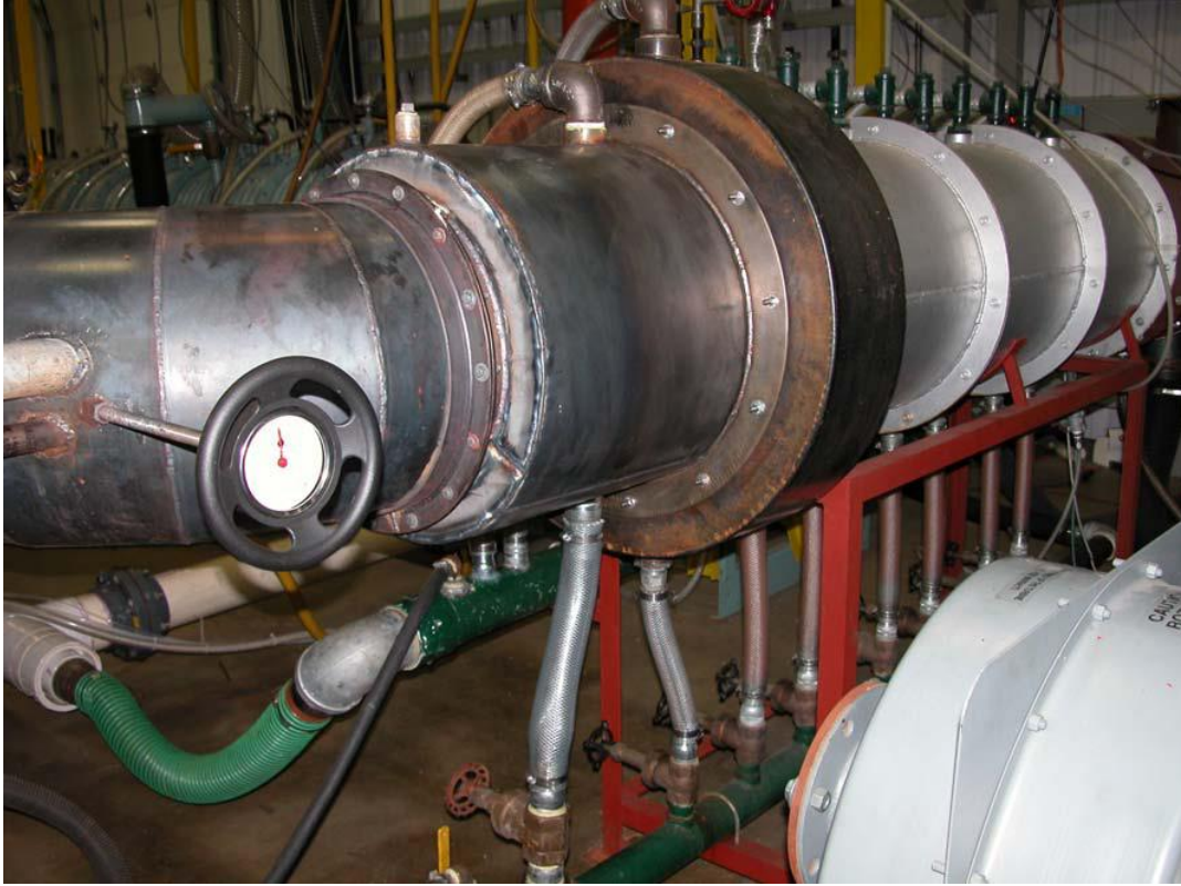
Figure 4: Auxiliary Combustor to Generate STEG
