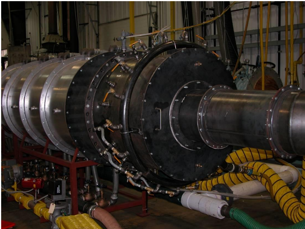
Figure 5: 7.5 million Btu/h Supplemental ULN Burner
