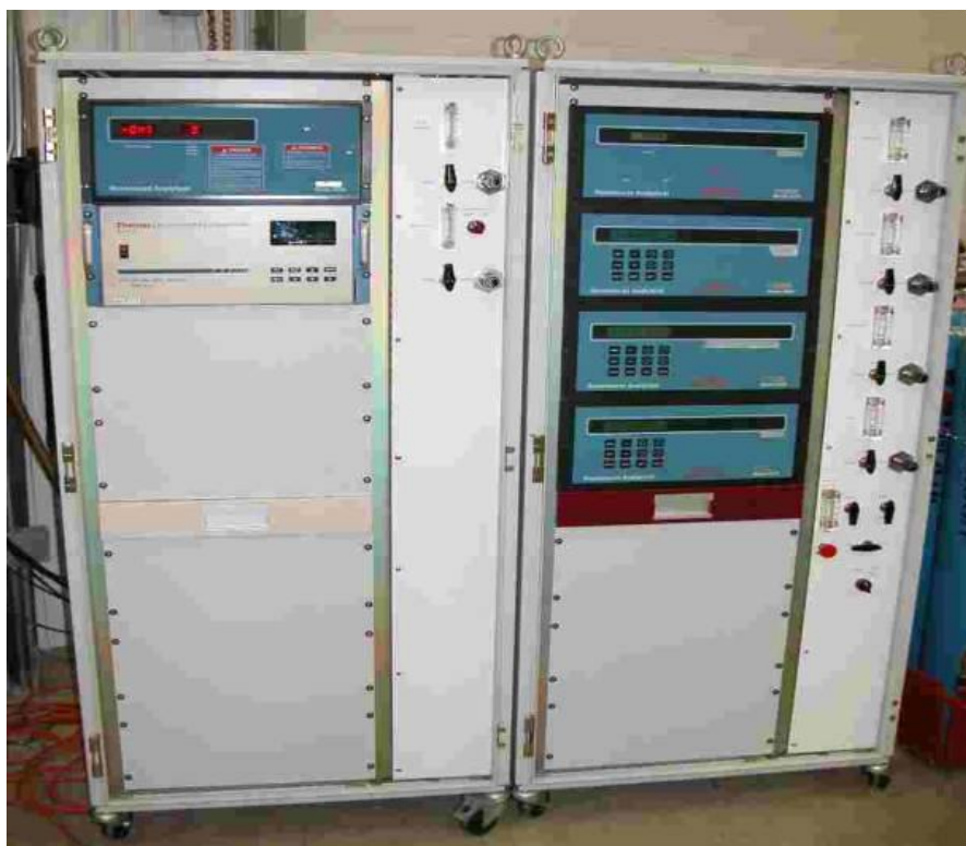
Figure 6: Panel Mounted Emissions Monitors
