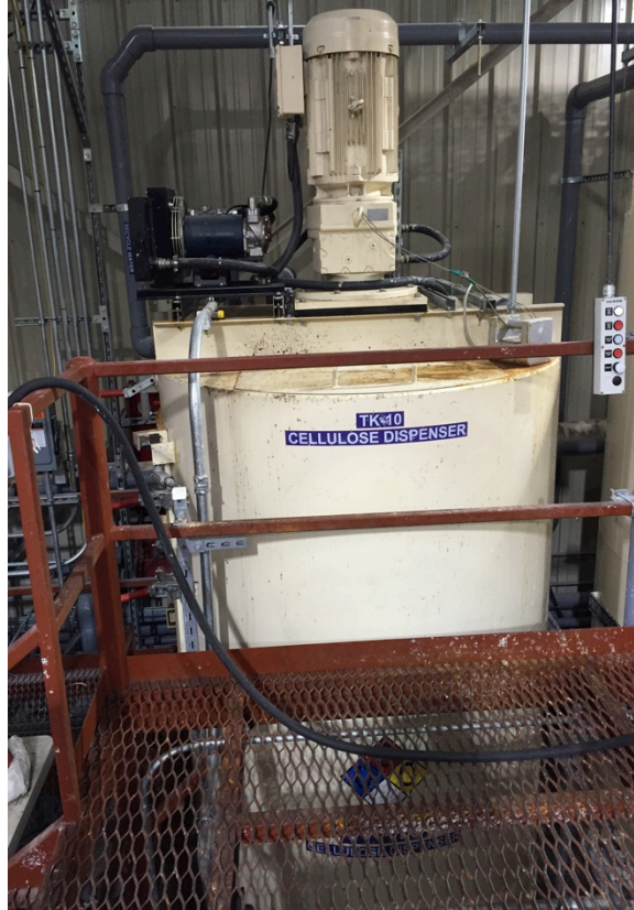
Figure 2-24 Cellulose Disperger used in the Fiber Cement Board Production Subsystem
