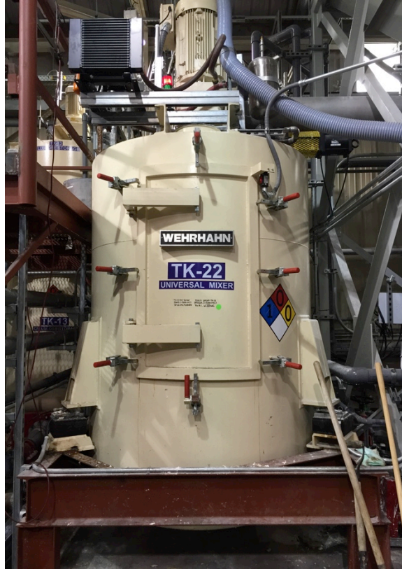
Figure 2-28 Universal mixer used to mix carbonate cement, refined cellulose slurry, recycled water and additives in preparation for feeding to sheeting machine
