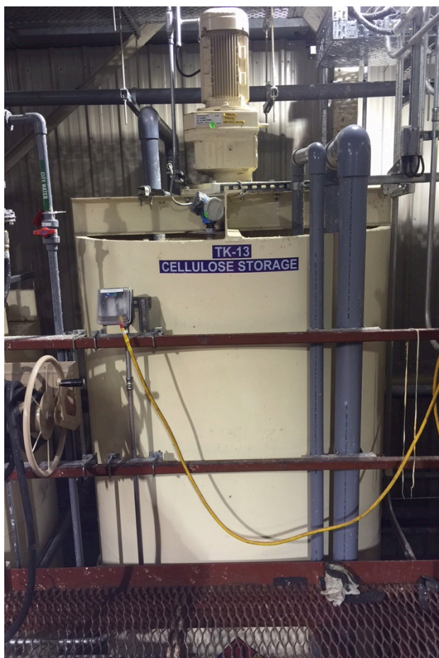
Figure 2-26 Cellulose Slurry Tank used in the Fiber Cement Board Production Subsystem
