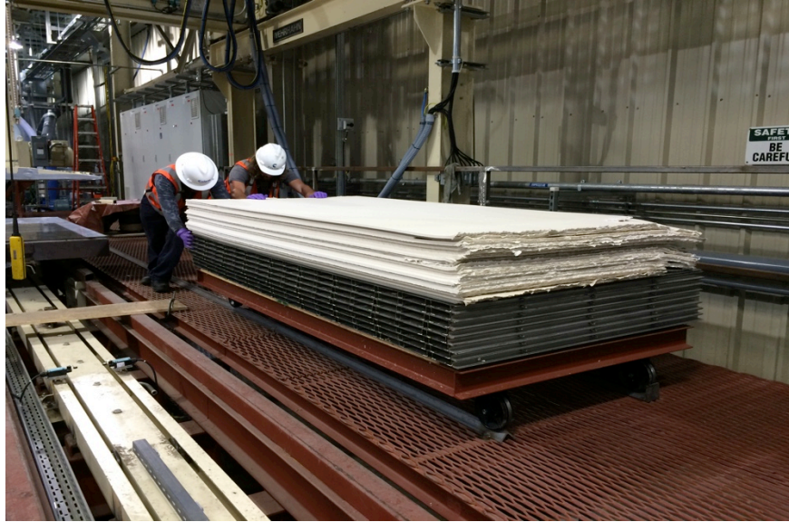
Figure 2-34 Calera carbonate fiber cement sheets stacked on the stacking cart moved by trolley into the pre-curing unit
