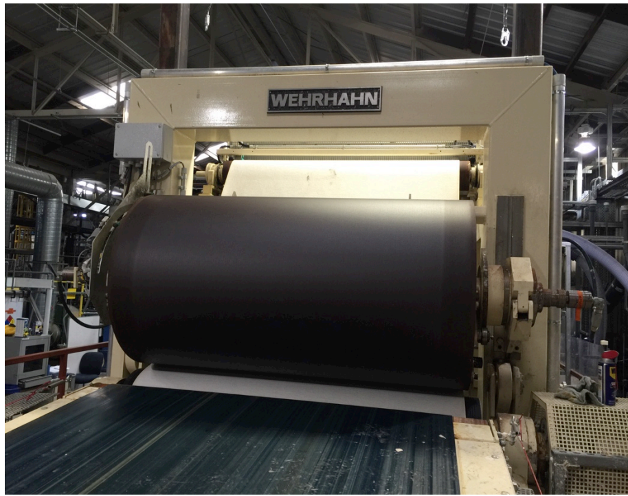
Figure 2-32 Accumulating forming roller on the Calera carbonate to fiber cement sheeting machine
