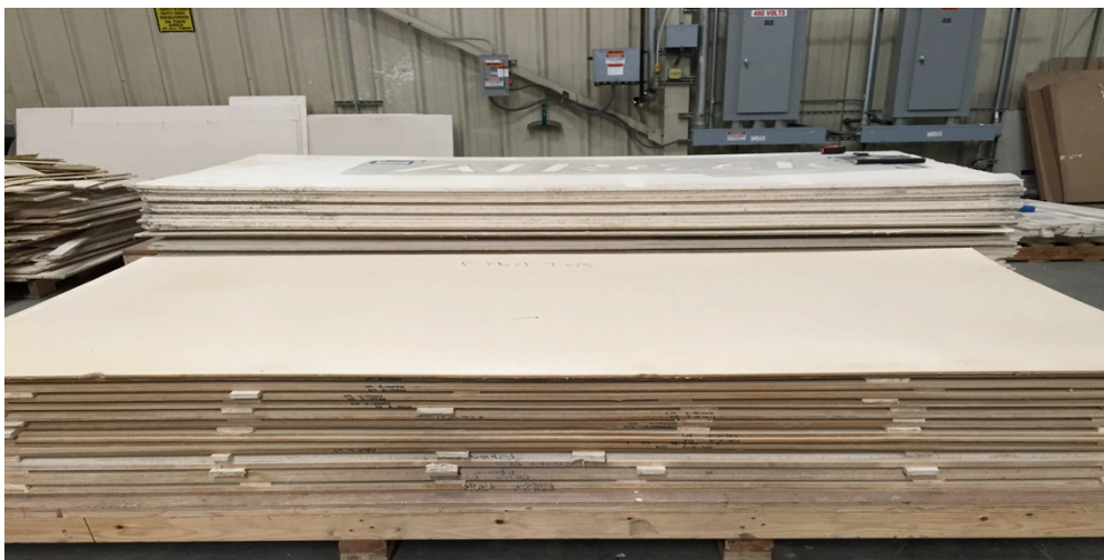
Figure 2-37 Fiber cement sheets stacked and packed onto wooden pallet after autoclaved
