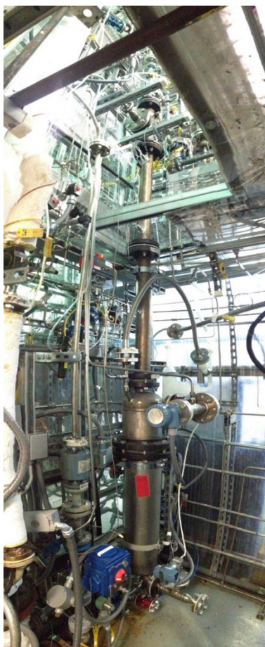
Figure 2-18 Distillation column used for separation of product from copper reagent
