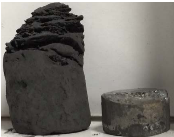
Fig. 23. Combustion products of Mo/Si/B/Ti mixture designed for 85% \text{Mo}_5\text{SiB}_2 and 15% \text{TiB}_2 . The left pellet was obtained by conventional SHS, while the right product was obtained by the chemical oven technique.
