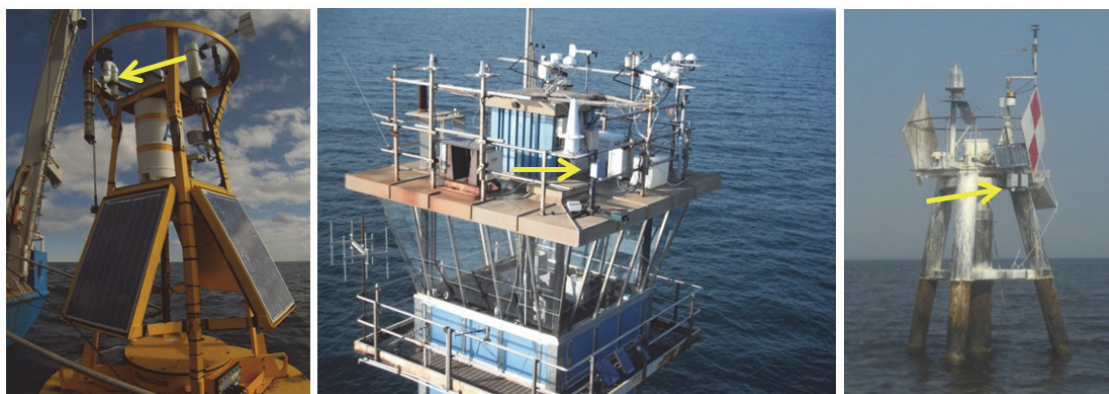
Figure 2-1. Examples of acoustic bat detectors deployed at offshore "structures" including NERACOOS Buoy A (left), the Chesapeake Light Tower (center), and Albermarle ATON (right). Yellow arrows highlight bat detector locations.
