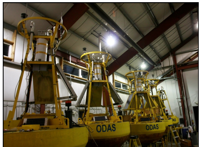
View of detector (in red circle) mounted on buoy (left) and a series of buoys with detectors installed, ready for deployment (right). The acoustic detector was deployed on the upper structure of a weather buoy deployed approximately 14.1 km off the coast of York, Maine.
