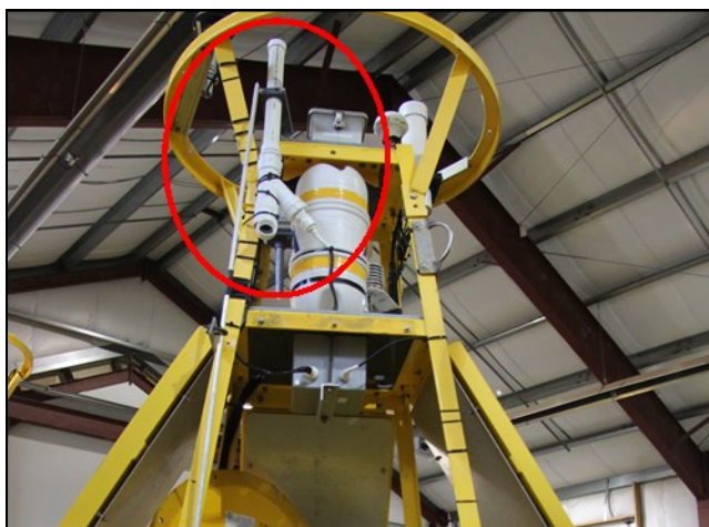
View of detector (in red circle) mounted on buoy (left) and a series of buoys with detectors installed, ready for deployment (right). The acoustic detector was deployed on the upper structure of a weather buoy deployed approximately 14.1 km off the coast of York, Maine.
