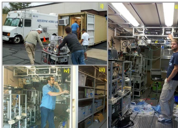
Figure 5. Instrument installation and packing at Aerodyne in preparation for seatainer shipment to India. Clockwise from upper left: i) installation of HR-ToF-MS in instrument seatainer, ii) Brett Palm - finished with all instrument installation, iii) all non-mounted instrumentation and supplies packed and catalogued for shipping/customs in non-instrument seatainer, and iv) Doug Day conducting final HR-ToF-AMS tests.
