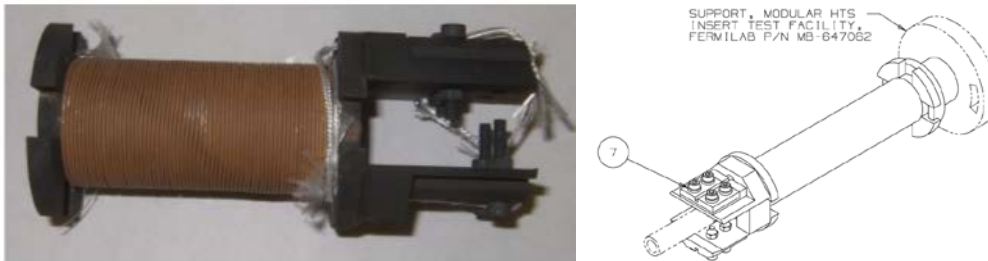
Figure 3: (a) The Inconel 600 coil former assembly designed and fabricated, with the 2-layer prototype coil after polymer burn off heat treatment and a 100 bar overpressure melt processing, and (b) a machine shop design drawing of the coil being mounted onto a high current coil test probe. The probe is capable of testing the coil with a current capability of 2 kA. The current leads were supported through Inconel 600 pieces that will latter on be replaced with Inconel 600
