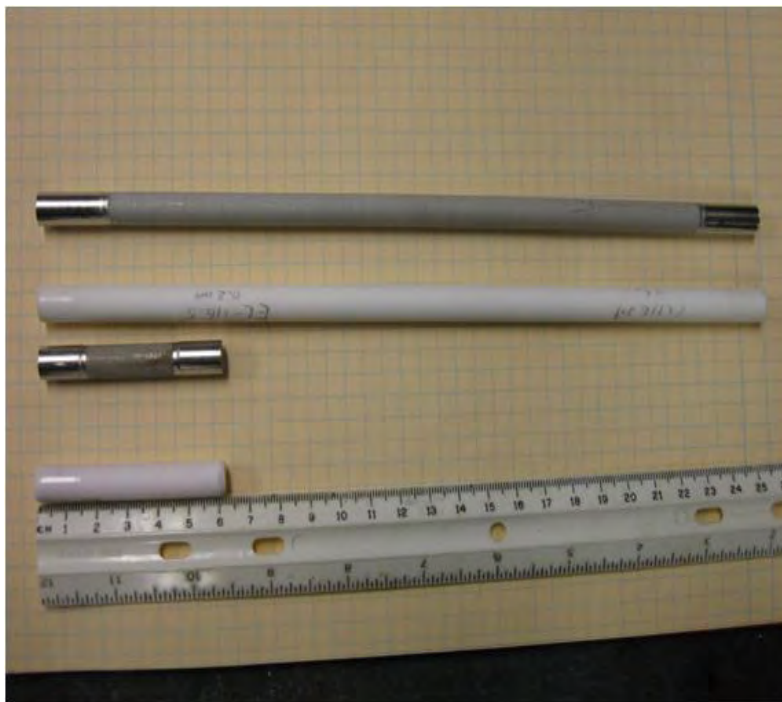
Figure 2. 6 cm and 25 cm long porous stainless steel supports (silver-gray colored) used to grow the membranes.
