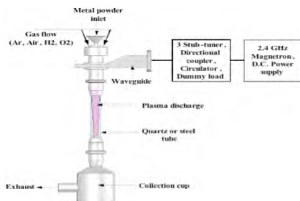
Figure 1. Schematic of AdEM's atmospheric plasma oxidation reactor for rapid oxidation of metal powders.
