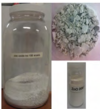
Figure 3. (a) SEM image of ZnO NW powders produced using the reactor shown in Figure 2. (b) The photographs of bottles containing ~250 grams of ZnO NW powder and 6 gms of ultrafine NW powder (~5-20 nm diameter; >20 microns length).
