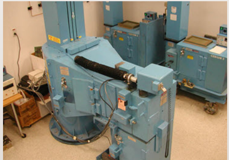
Gamma irradiation equipment for Hardness Assurance and qualification.
