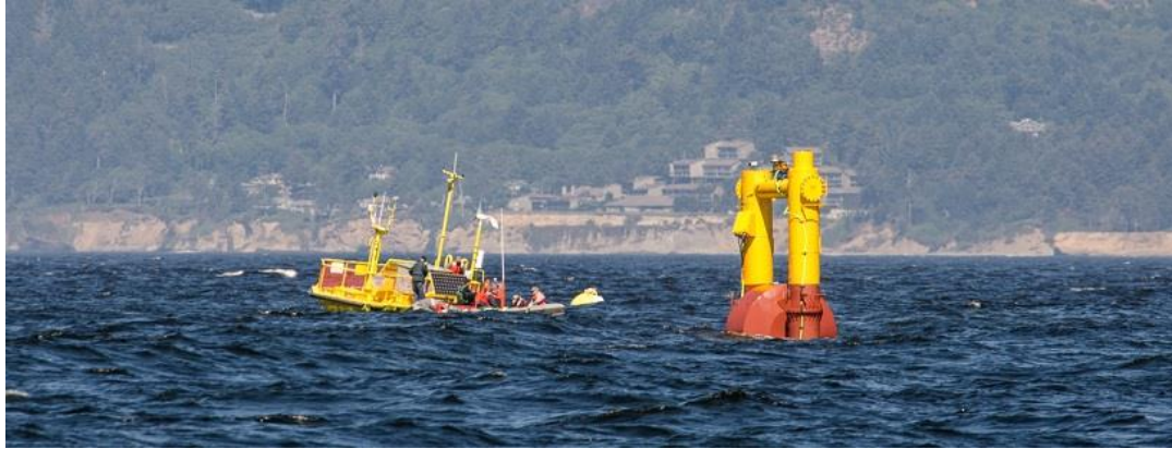
Figure 4 Deployment of the umbilical cable connecting the WET-NZ device under test to the Ocean Sentinel at NNMREC's open-ocean test site north of Newport, OR.
