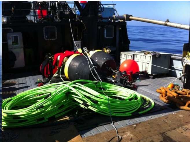
Figure 7 Recovered umbilical and corner-marker buoys.
