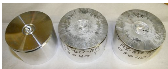
Figure 1. Anvils before and after thermal explosion of a liquid explosive; left was the pristine anvil; also shown are top anvil (middle) and bottom anvil (right) after the thermal explosion.
