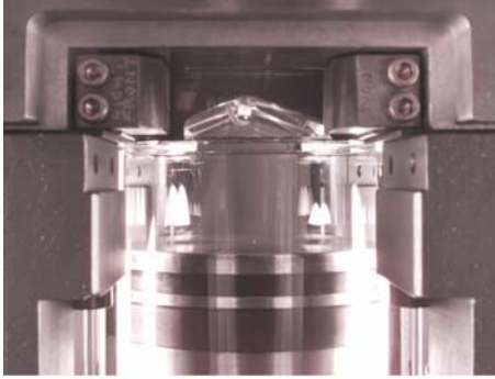
A homogeneous charge (port-injected) engine incorporating gable windows (Sandia National Laboratories)
