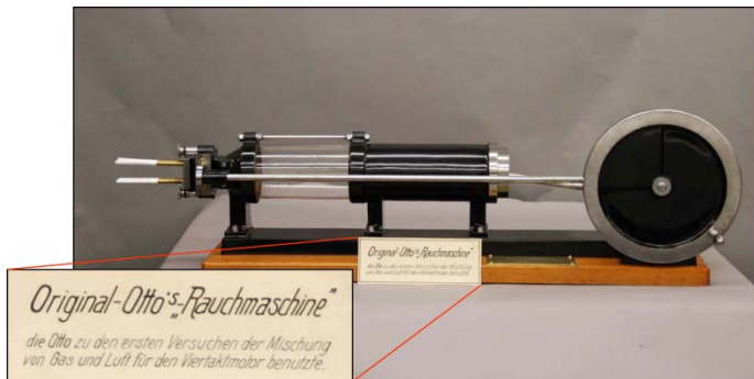
Figure 1. Nicolaus Otto's original "smoke machine". Photo courtesy of Bengt Johansson and Mattias Richter, Lund University.
