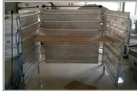
Figure 1 Experimental setup of radiant cubicle
