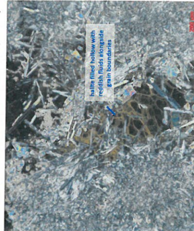
MB139 – Polyhalite/Anhydrite region after testing – sample 13079
