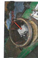
Samples can be added as a whole and intact chunk into the ball mill.
