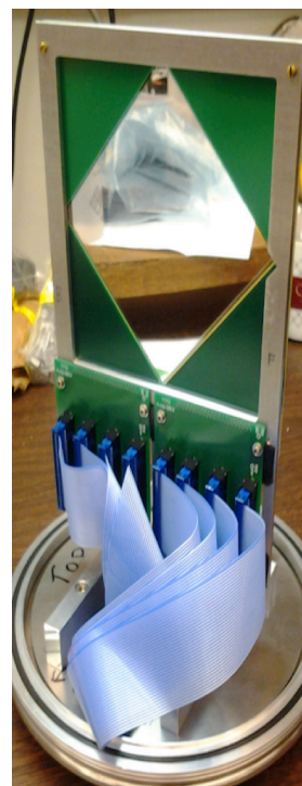
Figure 7: Left panel: A photo of the Micron Semiconductor Ltd. TTT2 type Si strip detector with the new PCB packaging funded by this award. Right panel: The detector on a mounting frame, attached to a standard vacuum flange. This configuration allows easy handling of detectors and minimizes the required cabling length. The box housing HINP motherboard and chips can be attached directly on the opposite side of the flange.
