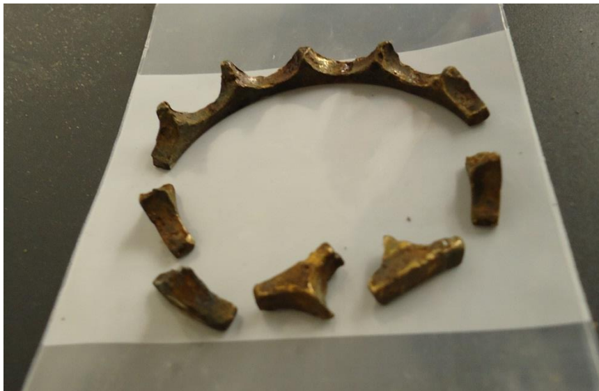
Figure 39. Pieces of shaft bearing cage removed from Frick RXF-15 compressor.
