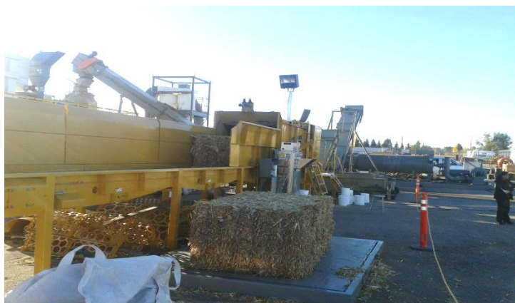
Figure 24. Hammer mill used at INL for grinding the feedstock
