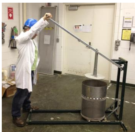
Figure 30. Manual basket packing device, designed and fabricated by MBI team
