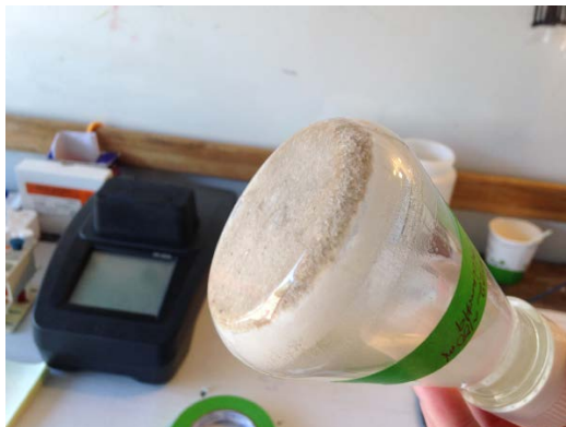
Figure A2. An unfiltered portion of the Mixing Zone sample #2 was mixed with calcium and growth-containing medium in a flask that contained unconsolidated 0.5mm (0.20 inch) quartz sand. After 24 hours of incubation, the sand was observed to be cemented to the bottom of the flask and the urea in the liquid dropped from 24 g/L to 6.6 g/L indicating ureolysis-driven MICP was observed with the field condition chemical combinations and a sample from the subsurface.
