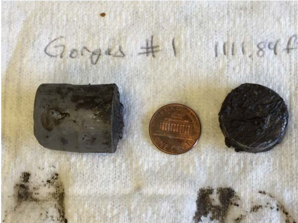
Figure 10. Side wall core collected at elevation 338.9 m (1111.84 feet) bgs (approximately 1.8 m) (6 feet) above the MICP sealed fracture). The interface between the steel well casing plug (right) and the one-inch cement plug (left ) contained a black, soft, mud-like material which was found to contain calcite.
