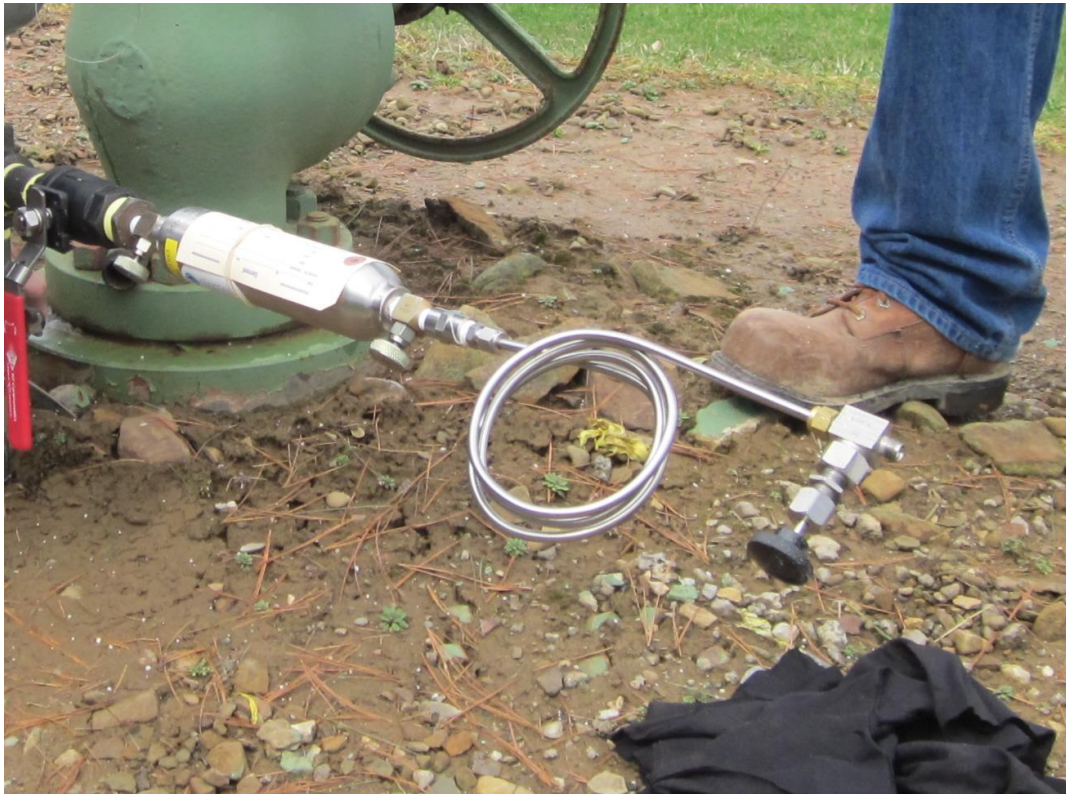
Figure 4-1. Collection of Annular Gas Sample at Test Well
