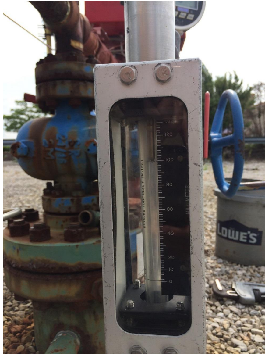
Figure 4-3. Flow Meter Used to Measure Gas Chamber Volume in Test Wells
