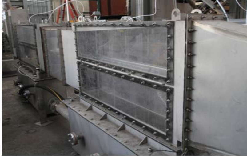
Figure 8: CARE NeuStream® FGD absorbers installed at the Drake plant
