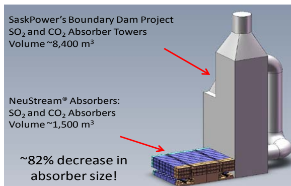
Figure 1: CO 2 absorber size comparison: 110MW (net) NeuStream ® vs. CanSolv's 110MW (net) SaskPower Boundary Dam Unit #3 project. Includes flue gas desulfurization (FGD), CO 2 and amine wash absorbers.
