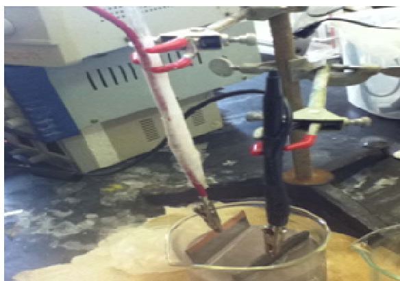
Figure 44: Setup for pre-treating the sintered nickel
