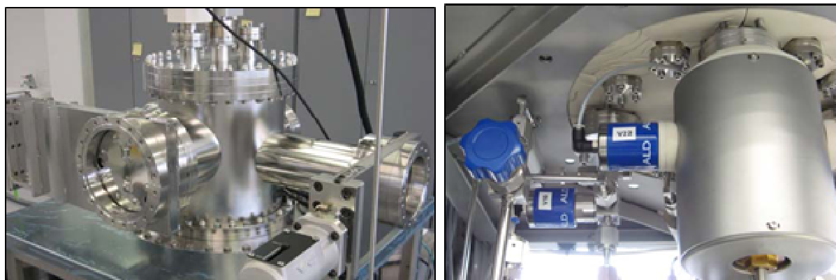
Figure 72: Photograph images of an ALD system under installation at SDSU to be used to grow dense and pin-hole free catalyst and protective layers.
