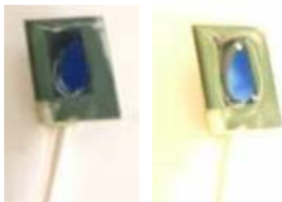
Figure 59: Electrodes made from a-Si solar cell material: electrodes where top layer is ITO (left) and electrode where Co 3 O 4 is deposited onto ITO (right);
