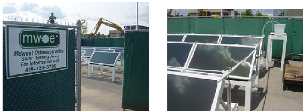
Figure 69: Outdoor testing center for superstrate type PEC modules and hydrogen collection setup.
