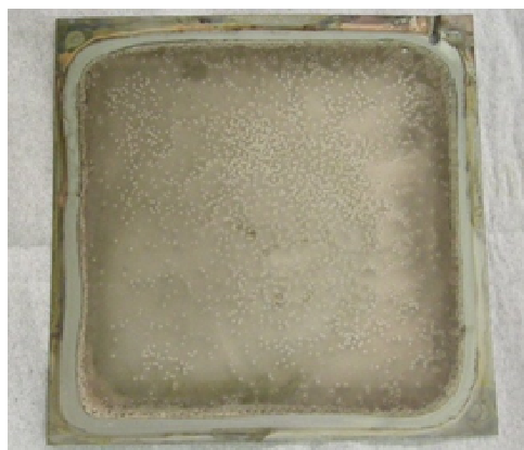
Figure 21: Electroplated porous Ni coating
