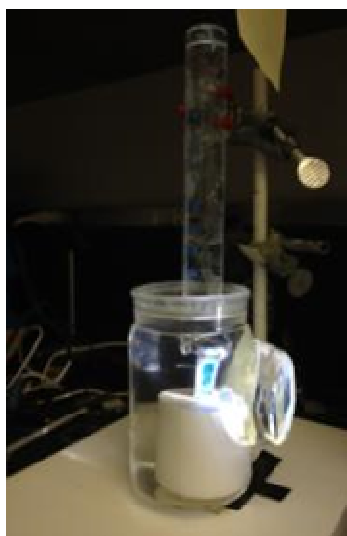
Figure 33: The experimental set-up for measuring the STH efficiency of the PEC electrodes;
