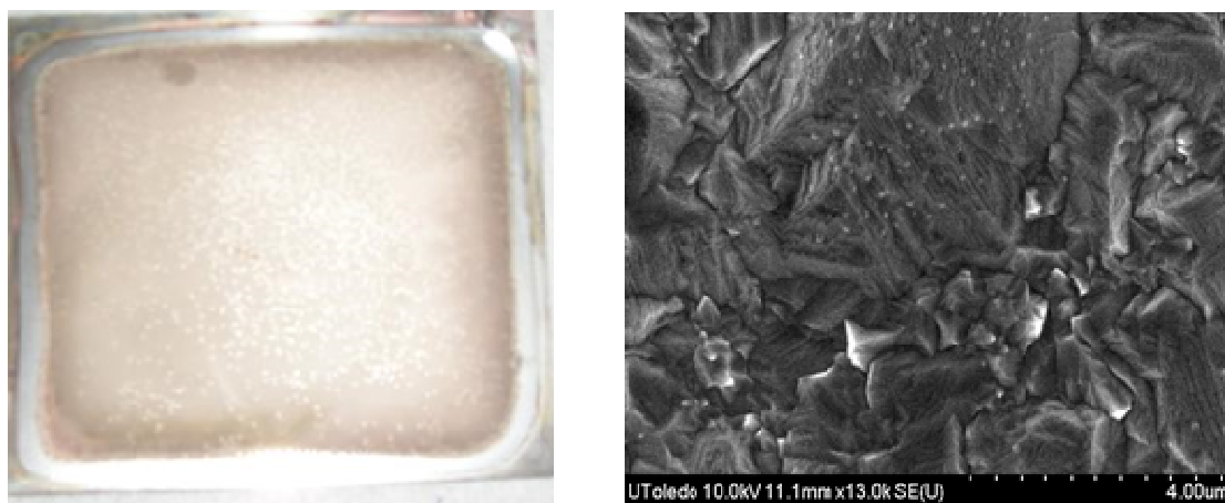
Figure 26: A picture (left) and a SEM image (right) of a porous Ni-plated electrode with (\text{NH}_4)_2\text{SO}_4 as precursor
