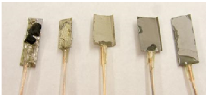
Figure 53: Electrodes made from hydrogen evolution catalysts (from left to right): sintered Ni, plated Ni ( \text{ZnCl}_2 precursor), plated Ni ( \text{NH}_4\text{Cl} precursor); plated Pt, etched stainless steel;
