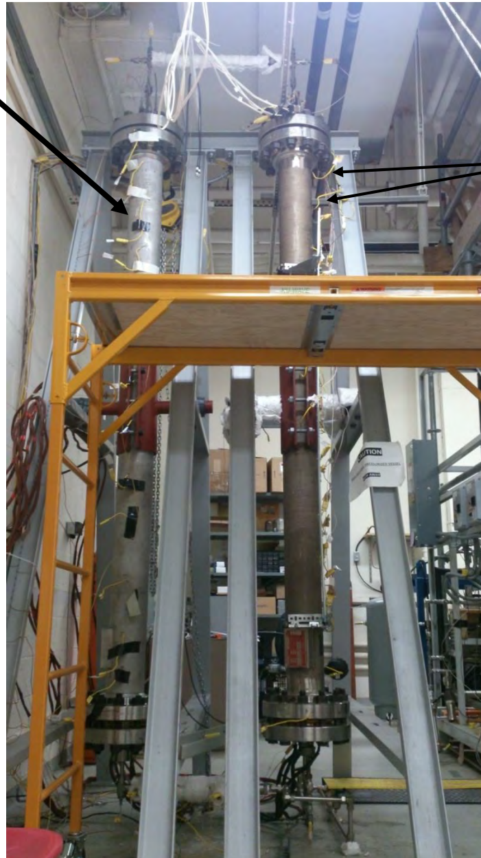
Figure A8. Second Pressure Vessel/Test Section Assembled on the Supporting Frame
