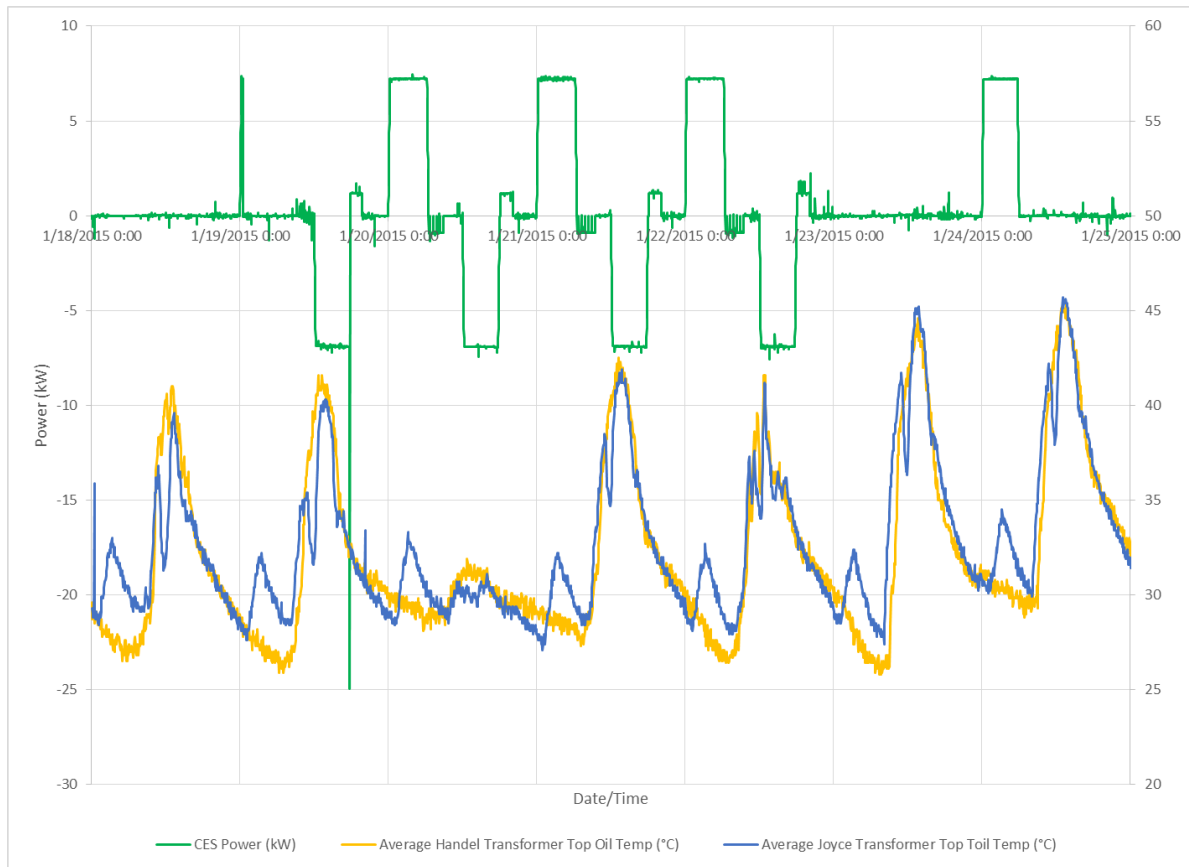
Figure 123: CES Power, and Average Oil Temperature of Both Windings for the CES and ZNE Transformers the Week of January 18, 2015
