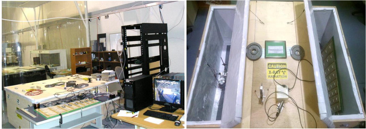
Figure 1.6: Left: GEM production and commissioning site at Fl. Tech. The clean room tent is visible in the background. Right: Test stand with x-ray generator on left and GE1/1 on right inside large shielding box.
