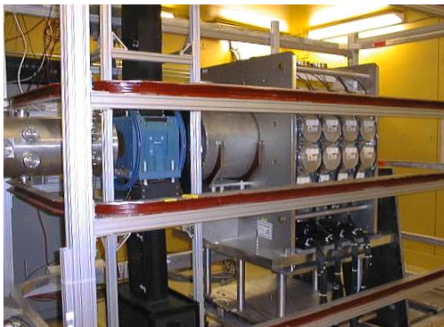
Fig. 16: Polarized ^3\text{He} neutron spin filter for the NPDGamma experiment at LANSCE. This polarizer worked on-line for this experiment over almost a year of continuous operation.
