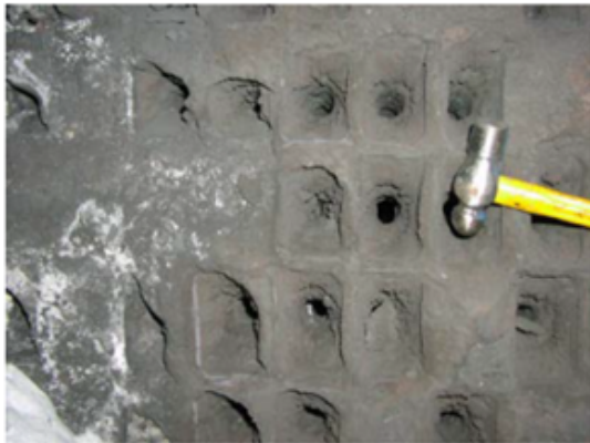
Figure 1. Examples of tube sheet fouling at Wabash River IGCC plant (left) [Guenther et al. 2011] and Polk Station IGCC plant (right) [McDaniels and Hornick, 2002].
