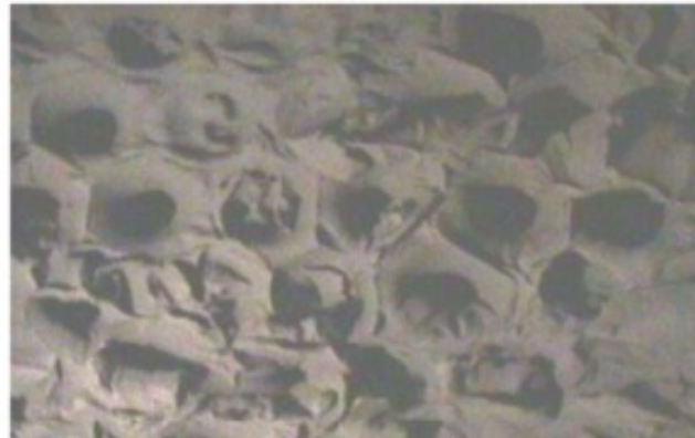
Figure 1. Examples of tube sheet fouling at Wabash River IGCC plant (left) [Guenther et al. 2011] and Polk Station IGCC plant (right) [McDaniels and Hornick, 2002].
