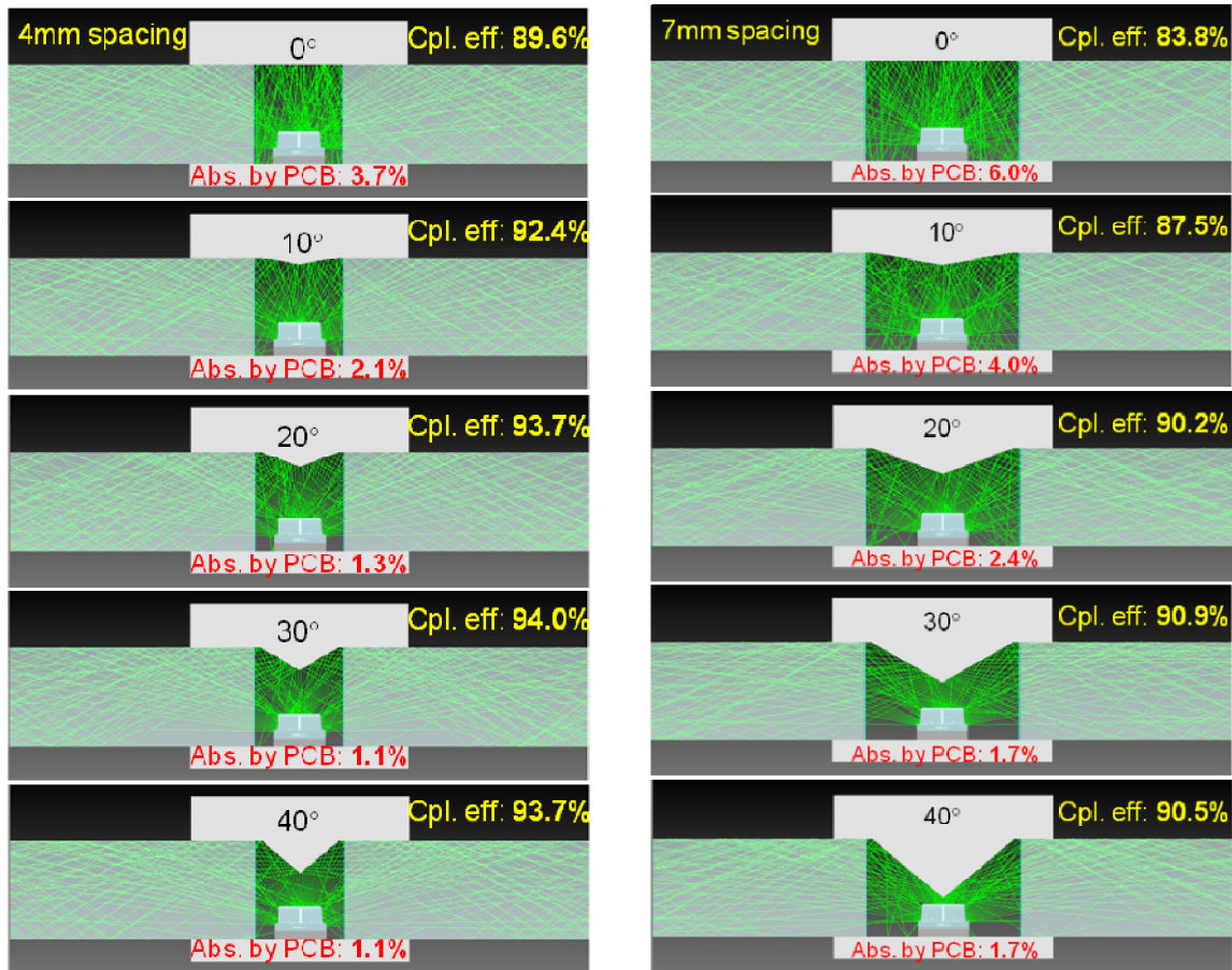
Fig. 27. Ray-tracing simulation of the light coupling from an LED into lightguide edges with two different cavity widths (4 and 7mm) and reflector angles (0-40°).
