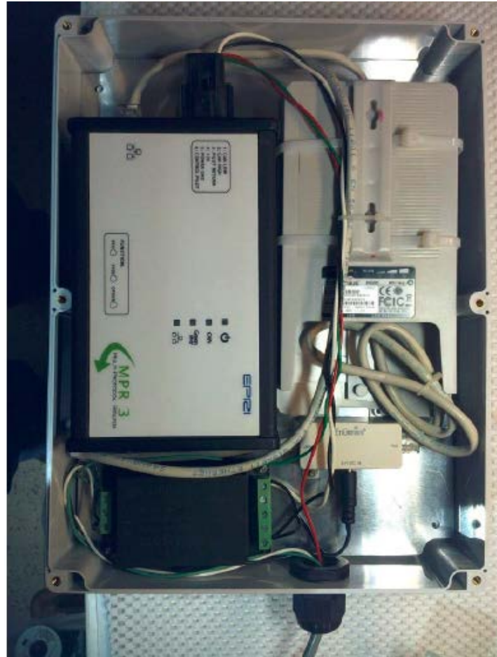
Figure 5-14 Electric vehicle supply equipment communication box layout and contents
