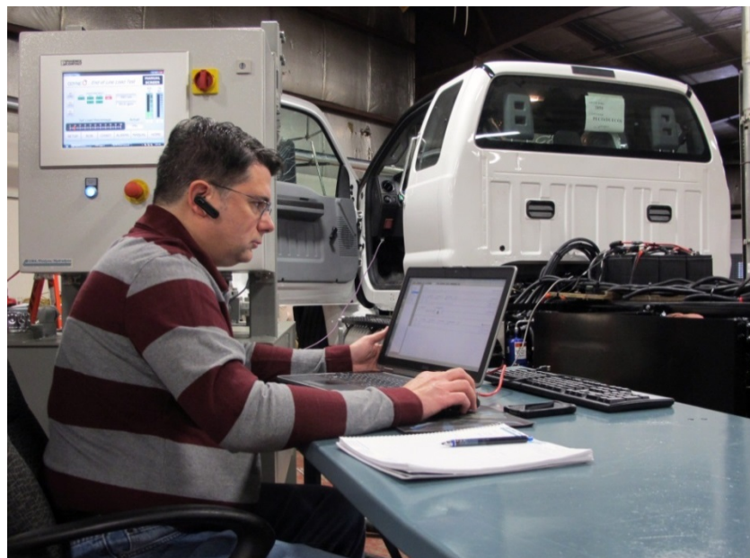
Figure 3-22 Using the automatic tester for testing the final assembled hybrid system
