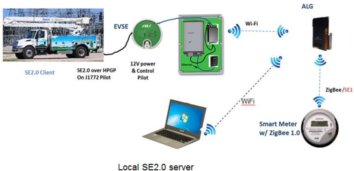
Figure 5-8 Single plug-in vehicle communication architecture
