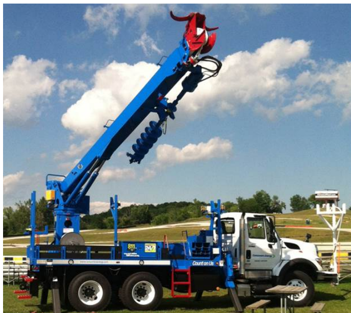
Figure 3-18 Final configuration as a digger derrick
