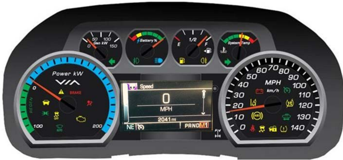
Figure 4-8 Pickup truck dashboard display
