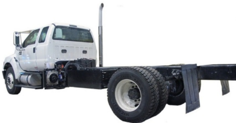
Figure 3-17 Chassis with hybrid system installed
