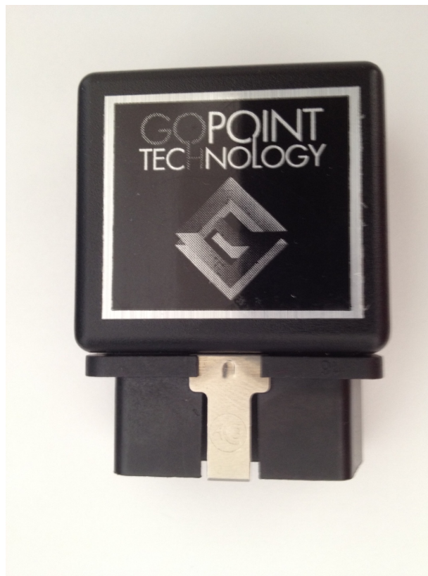
Figure 5-2 Controller-area network bus hardware interface module
