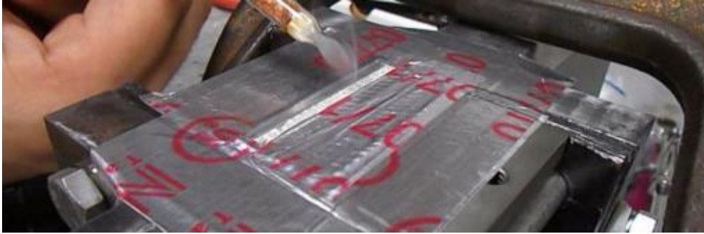
Figure 37: Shown is the leak checking process. The hot channels were sealed into the rig with a vacuum being drawn, and the cold channels were exposed. All but one row of the cold channels were masked by impermeable tape. As the vacuum was drawn on the hot channels, a smoke wand was passed over the exposed cold channels. The smoke is shown being drawn into the channels, indicating a leak between the hot channels and this row of cold channels.
