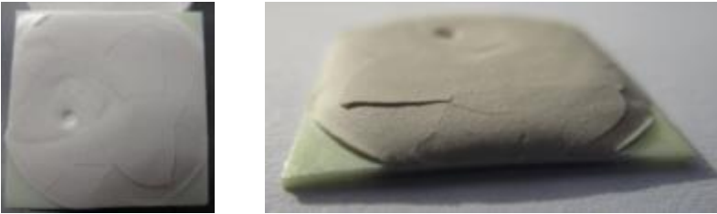
Figure 16: Mullite from pellet adhered well to ZrO 2 ceramic tape after firing showing good compatibility.
