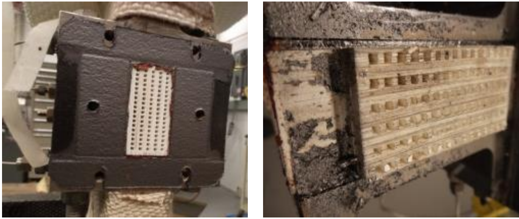
Figure 40: DFB prototype after testing showing the part handled the aggressive test conditions.
