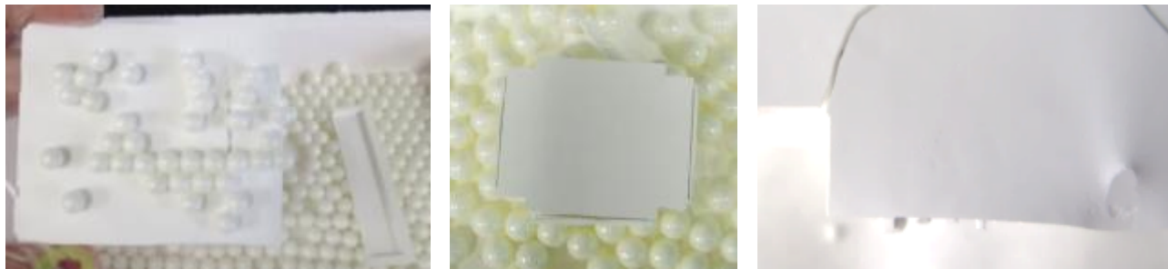
Figure 21: Results of mobile media bed experiments. (Left) Small media bed – sample bottom with cracking and media sintered to sample. (Center) Large media bed – full size part. (Right) Close up of B bottom – dimple in lower right shows where the media adhered to the part.
