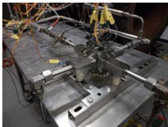
Figure 36: HX performance test rig with instrumentation
