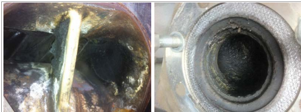
Figure 84. Inspection of Dry-Screw Compressor Originally Installed on MTR's 1-TPD System
